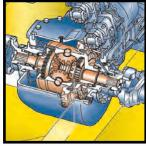
truck is travelling, thereby boosting productivity. In addition, the differential lock switch, which is a three position switch, can lock up the rear axle differentials only, or all axles for maximum performance in the worst conditions.
