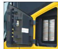
External air conditioner filter
