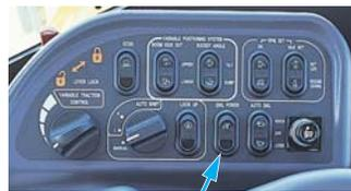
Dual mode engine power selection switch
