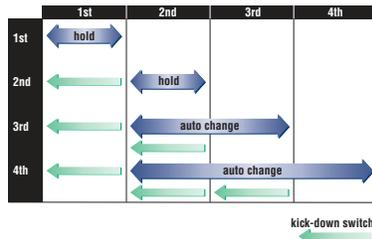
downshifts from second to first when beginning the digging cycle. It automatically upshifts from first to second when the direction control lever is placed in reverse. This results in increased rim pull for better bucket penetration and reduced cycle times for higher productivity.
