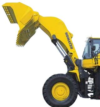
The WA600 can load 60 ton (70 short ton) trucks with the standard boom. The WA600-3 required an optional high lift boom and 6.4m<sup>3</sup> 8.4 yd<sup>3</sup> bucket. The WA600-6 maintains good visibility for loading because of increased operator cab height.
