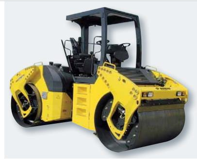
Safety: operator's position with rail and ROPS/FOPS.
