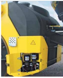
High capacity tanks for less filling stops; two pumps.
