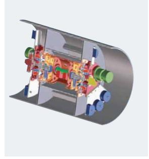
Drum with directed oscillation for ASPHALT MANAGER 2 (BW 190/203 AD-AM 2).
