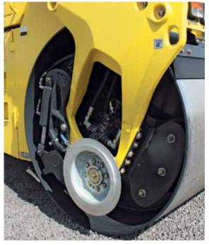
Efficient edge work with a cutting disc or pressure rollers.
