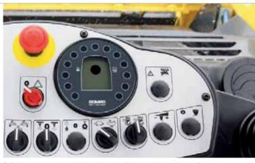
Safety: emergency stop switch and warning lights are arranged centrally.
